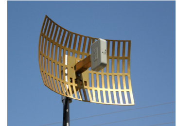
Antenna Mounted Vertically Polarised
